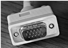
FIGURE 287. VGA video connector
