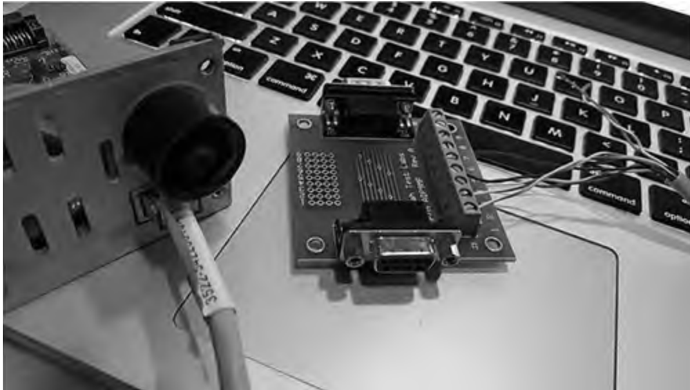
Figure 25-6 Final setup for RS-232 connectivity
