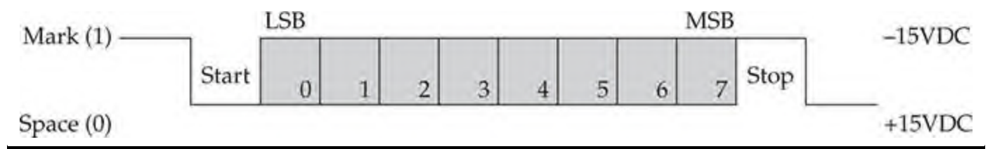
Figure 25-1 RS-232 waveform example
