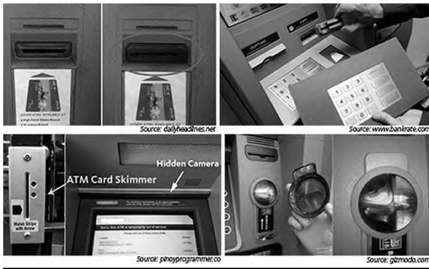
Figure 20-6 Skimmers attached to ATMs
